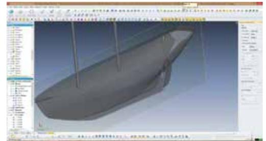
Image 8: Final Hull, Deck and Transom Surfaces
