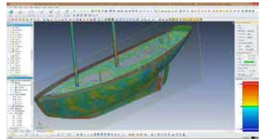
Image 9: Accuracy-Analyzer™ view showing the spatial distance between the mesh and generated surface
